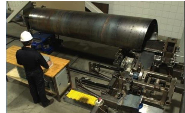
Keystone Tower Systems, Inc. in-situ tapered tower manufacturing
